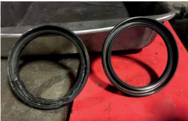
The old seal (on the left) lost its tensioning spring (which you can see in the catch pan) upon extraction; the fresh seal's spring is still in place.)
