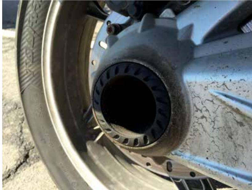
Dirty final drive showing signs of leakage.
