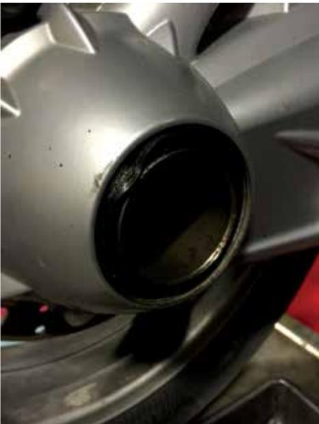
As the seal comes free, you may see that you've torn the edge of it. This is okay – it's better to tear the leading edge than to punch clean through.
