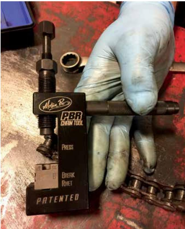
PBR ready for action in Break mode, with detachable handle in place.
