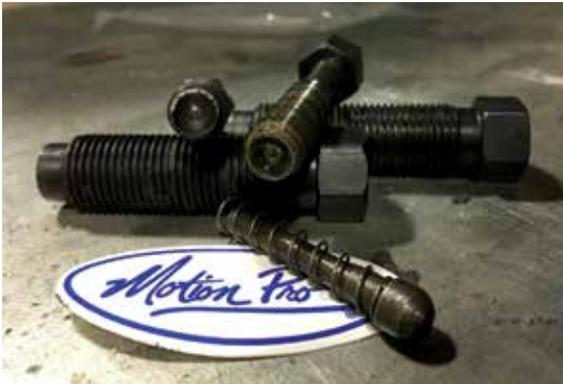
Extractor bolts on top of body bolts. Note broken tip of left extractor bolt. Extractor pin/spring in foreground.
