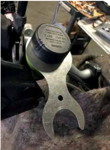
Using the BMW special tool to get into your brake and clutch fluid reservoirs makes the task easier and less prone to accidental damage to the components. At \$18.48 as of this writing, it's a small investment that could save you money in the long run.
