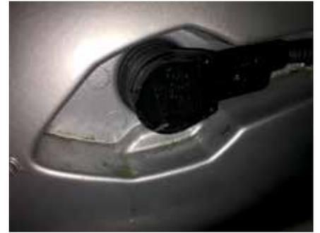
Fresh oil on the ground is never a good sign, but in this case it was a minor issue. Oil leaking out from the ignition coil tunnel generally points to an improperly seated donut gasket. Rotate the gasket (replace if it's damaged or torn) and try to get the cylinder head cover on correctly again. It sometimes takes me three or four tries.
