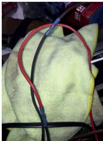
...and a butt-spliced crimped connector to make the wire long enough to reach the Fuzeblock. Crimped connections are easier to do (provided you have the right tool and connectors) than soldered connections. They're not necessarily better than soldered connections, but they are easier to repair on the side of the road if necessary.
