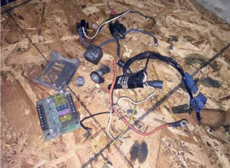
**Above**, All the removed components. **Right**, The aux socket connector – theoretically waterproof but obviously not actually so.
