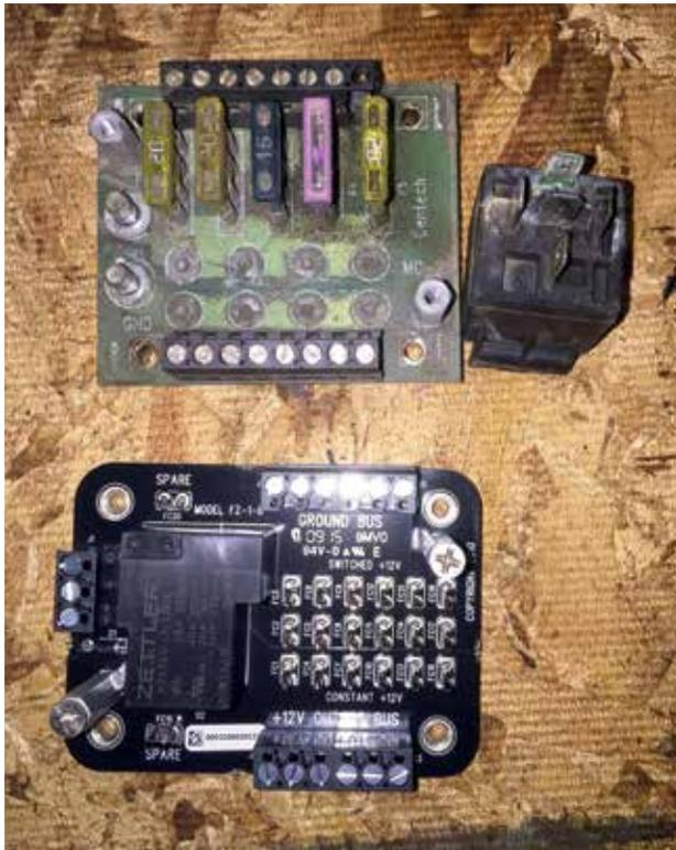
The old Centech (top) and new Fuzeblock units. Note the fried terminal at the top right of the Centech and the corroded terminals on the old relay.
