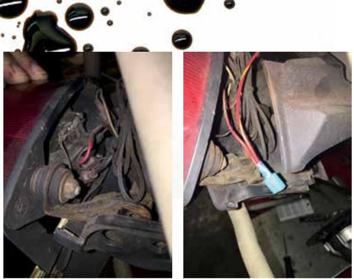
Removing the entire tail light assembly isn't necessary, but you do have to take out the mounting screws and drop it down to get access to the wires.
