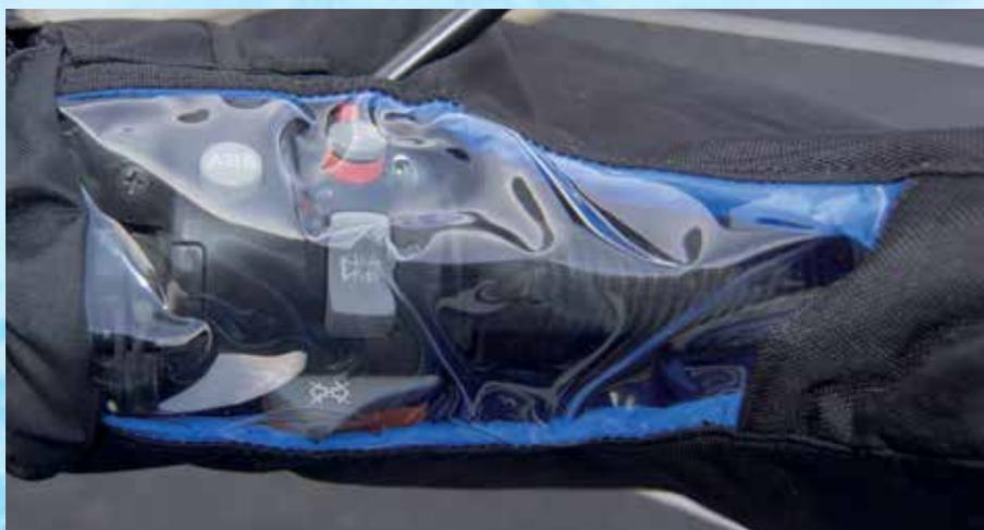
First and foremost is the clear plastic window that allows the rider to see both sets of handlebar controls. We all operate our motorcycles on muscle memory most of the time, rarely looking for the high-beam or horn button, but not being able to see those controls at all can be disconcerting to some riders. The windows in Wunderlich's muffs stay clear and pliable down below freezing, enabling quick looks to reassure riders where their controls are.
