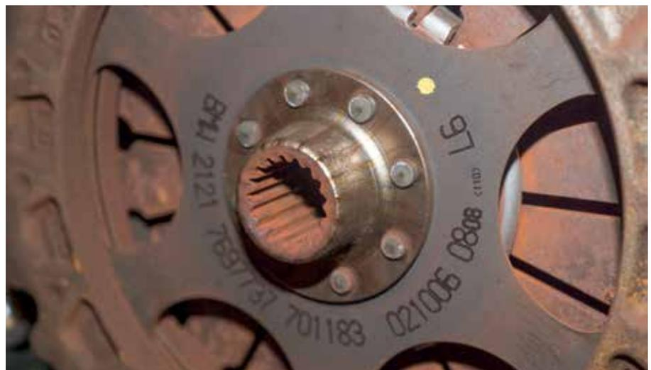
The rusty splines of the old clutch plate (aka friction disc).
