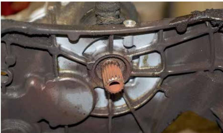
Rust on the transmission input shaft splines.
