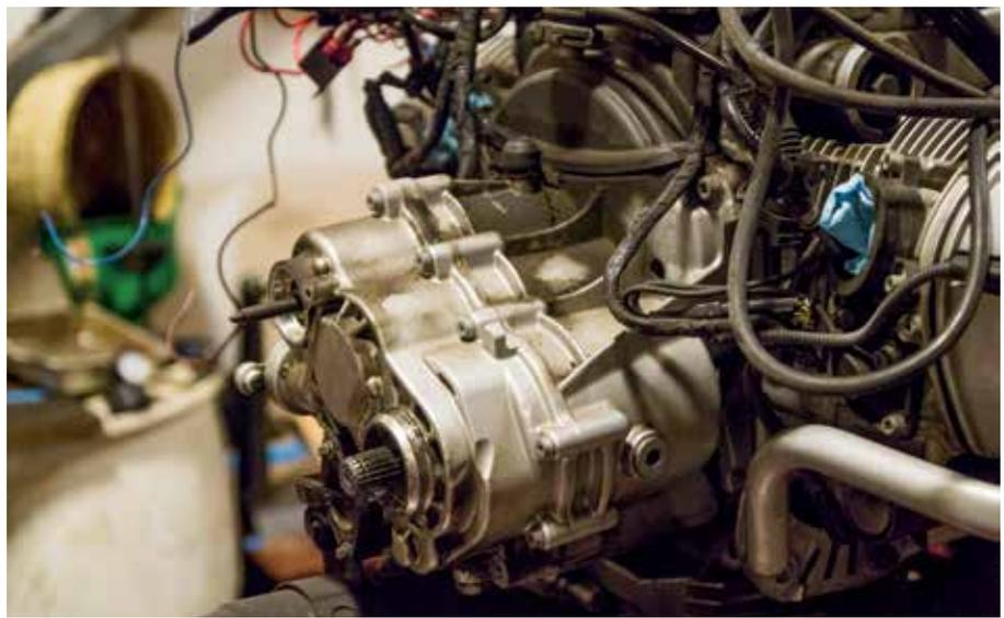
The transmission is dirt – dirtier than it should be, especially on top of the housing. This is an early indicator there may be problems inside the case. Note the pushrod extending from the top left of the transmission. The splined shaft at the bottom right of the housing is where the drive shaft connects to the final drive.
