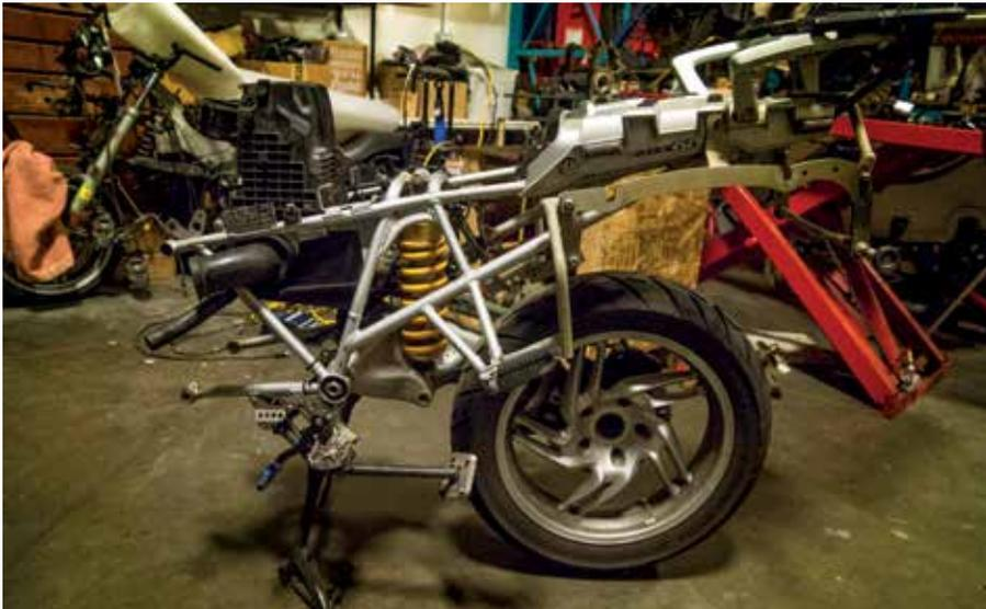
Leaving the rear wheel attached to the final drive allows for easy maneuvering of the entire rear section once it's disconnected.
