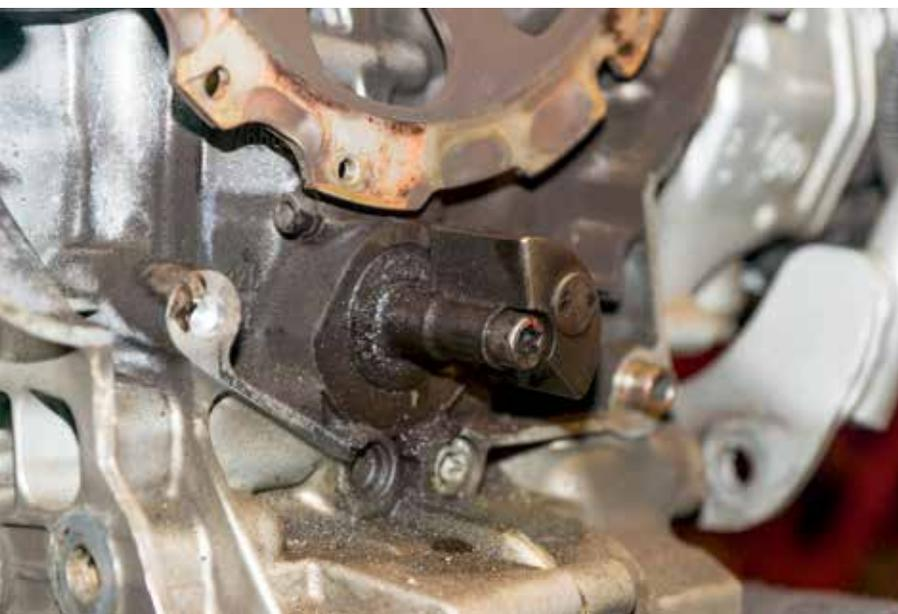
Engine oil being forced past the counterbalance shaft seal created a slimy, gloppy mess inside the space between the engine and the transmission.
