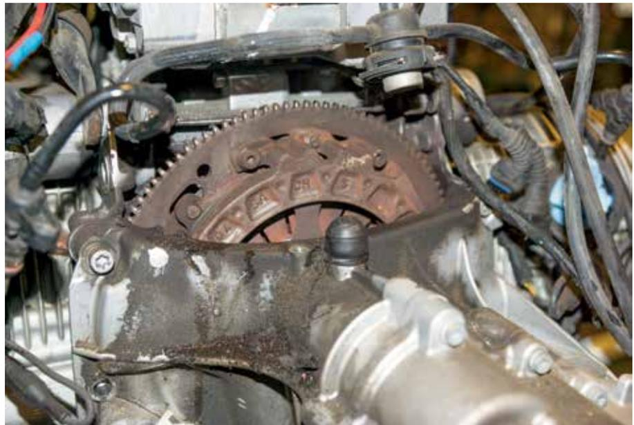
My first look at the rusted clutch components. While a certain amount of corrosion and wear – and possibly a bit of rust as well – is to be expected, this much rust is indicative of some hard water crossings during the bike's life.
