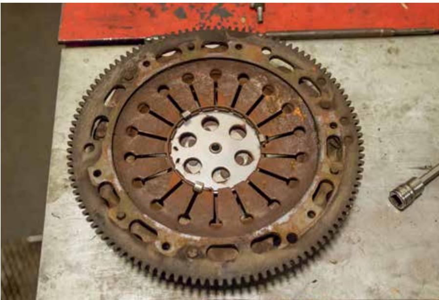
The rusty clutch spring plate that's part of the pressure plate assembly, which engages with the teeth of the starter motor. The protruding pins near the teeth are rivets that hold flat springs onto the other side of the assembly.
