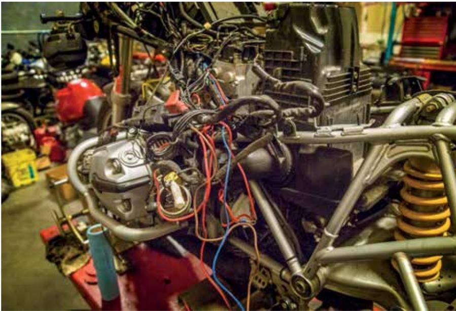
This rat's nest of wiring made things troublesome in the disassembly process. We disconnected, cleaned up and rerouted most of this during reassembly.
