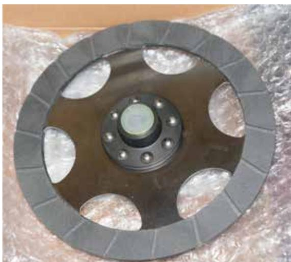
Siebenrock's oil-resistant clutch plate (imported by Wunderlich) is an easy upgrade that costs about the same as the OEM part. In operation, it has a slightly more positive feel than the stock disc.
