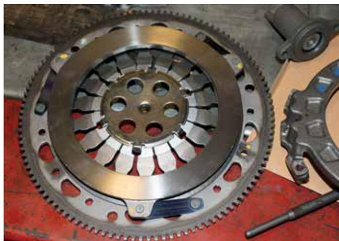
Pressure plate. This is the side that mates against the clutch plate; the hole in the center is where the pushrod goes. It pushes against the circular spring, releasing the pressure against the clutch plate and allowing it to spin freely, which is why you can shift gears.
