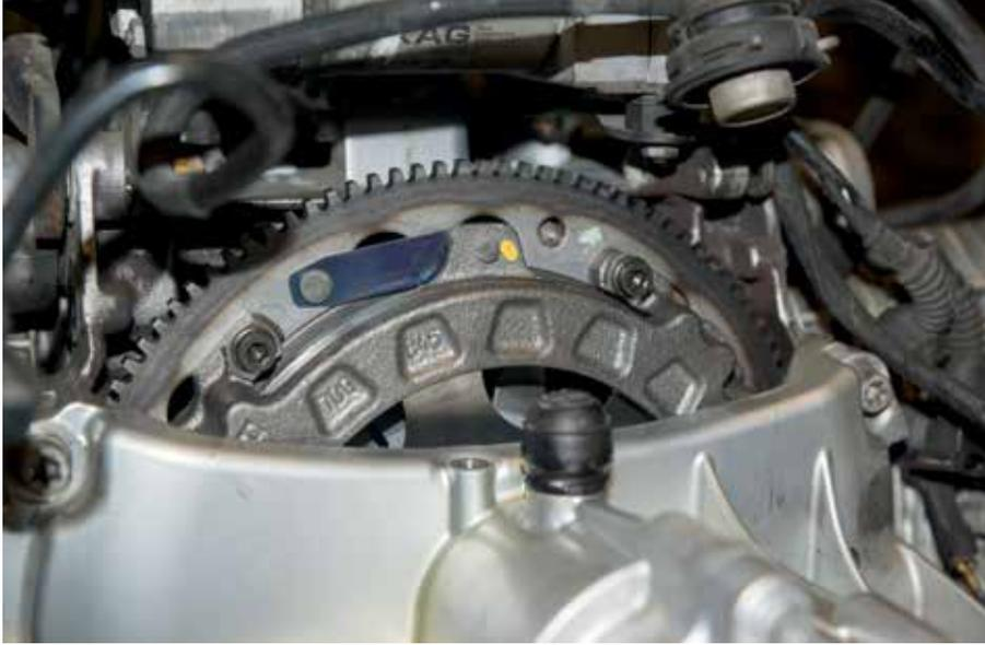
The clutch assembly is bolted onto the flywheel and the transmission is back in place, ready for the clutch cover to be installed. Note how clean everything is!
