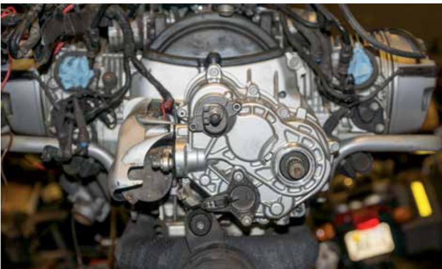
Ready to finish the reassembly. Putting the starter cover on at this stage makes it much easier to attach than if you wait until the back half of the bike is back in place. Note the gear shift potentiometer at the bottom of the transmission – this is what tells your bike's computer what gear you're in. It's plastic and costs \$219.40 to replace, so be careful not to damage it when you're moving the transmission around.
