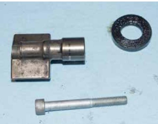
One bolt connects the counterbalance weight to its shaft; the seal keeps oil inside the engine, where it belongs.
