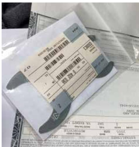
The special release tool for clutch and front brake master cylinder covers. It is BMW part number 83 30 0 402 038 and costs about \$15. Any BMW dealer can order one for you
