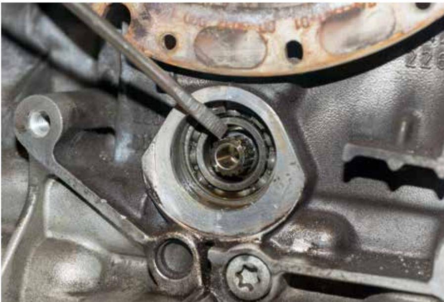
You can't install the counterbalance weight incorrectly. The screwdriver points to an extra-wide tooth that marries up to an extra-wide slot on the shaft.
