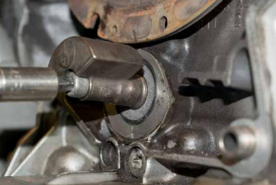
The counterbalance shaft seal and weight in place. Be sure to look up all torque values and use a quality torque wrench to secure all fasteners.
