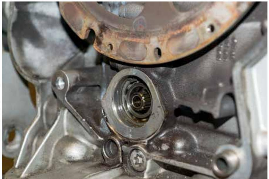
Tip the engine forward to keep oil from gushing out if you have to remove the counterbalance shaft seal. Wipe clean all mating surfaces and anything else you can get at with a rag.
