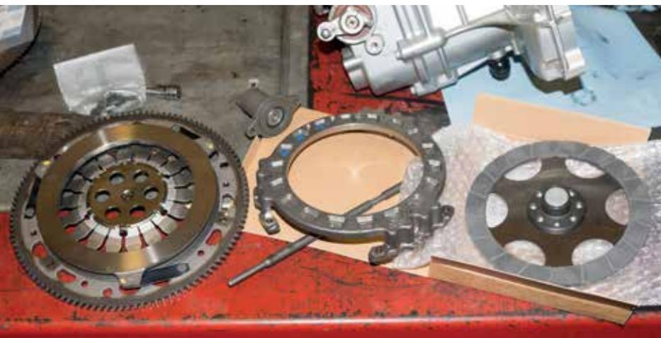
Shiny new clutch components – pressure plate on the left, housing cover in the middle and Siebenrock oil-resistant clutch plate on the right. The new pushrod is under the housing cover and the new slave cylinder between the pressure plate and housing.
