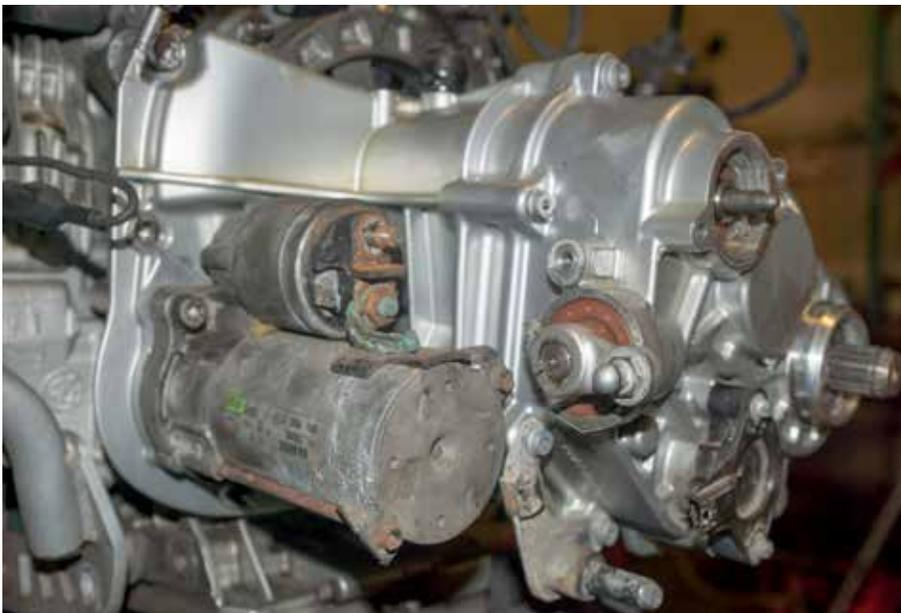
Next to the spanking-clean transmission, the starter looks positively disgusting. Be sure to clean any corrosion or rust from the electrical connections – hit them with sandpaper, steel wool or a wire brush to ensure the mating surfaces are fully clean.
