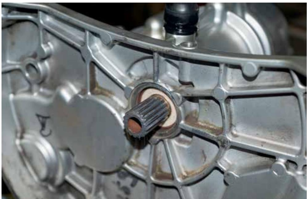
Splines of the transmission input shaft, cleaned and lubricated. Note the clean, fresh seal. Molybdenum-infused grease goes on these splines, but not in huge quantities, so be sure to wipe off any excess. You don't want to start your new clutch's life with a bunch of goeey moly paste slinging around inside the housing and possibly contaminating the friction surfaces.
