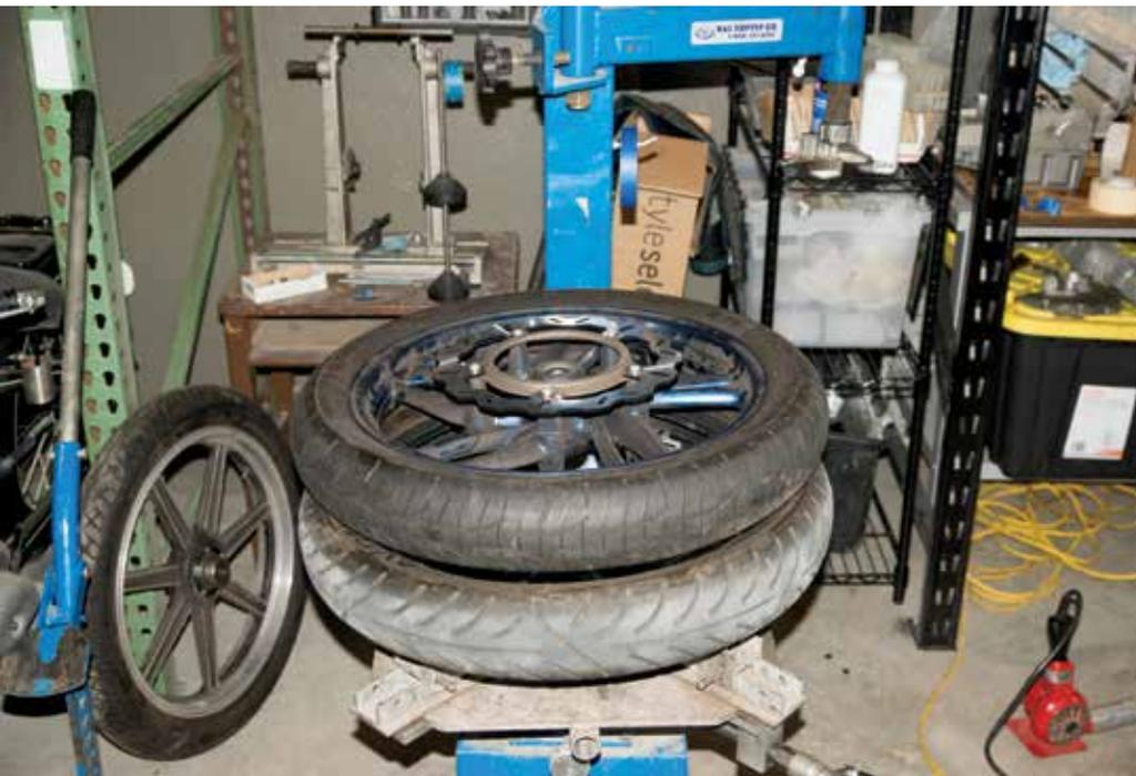
Use an old tire to make a stand for working on your front wheel. Avoid putting the brake rotors directly on a hard surface such as a metal work table or concrete floor.
