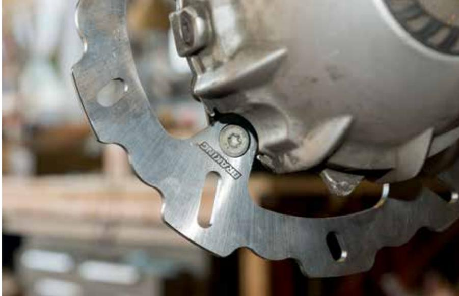
The cutout on the final drive makes accessing the rear brake rotor bolts one at a time possible, but it's a tight fit. Using a standard (short) T40 bit could result in stripping out the heads of the bolts.
