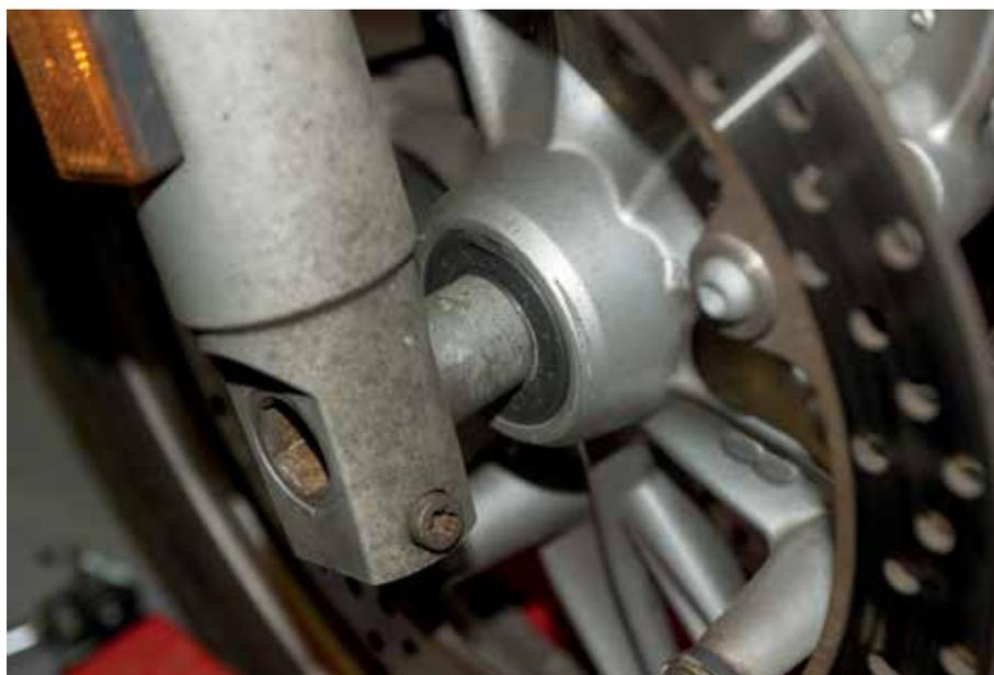
Inspect, clean and replace rusty components and again, pay attention to what order the parts are in when they come off. ALWAYS use a torque wrench and look up the torque specifications for things like the fork pinch bolt and front axle, shown here.
