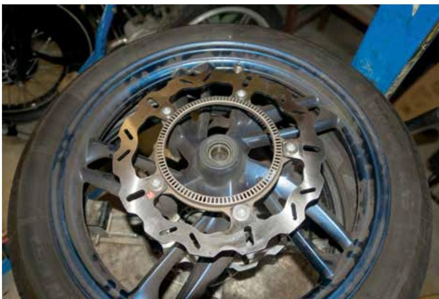
Installation is the reverse of removal, so pay close attention to the order of the components. Mixing up where the ABS sensor ring goes could adversely affect the functioning of your ABS unit. Even what order the washers are in is important.
