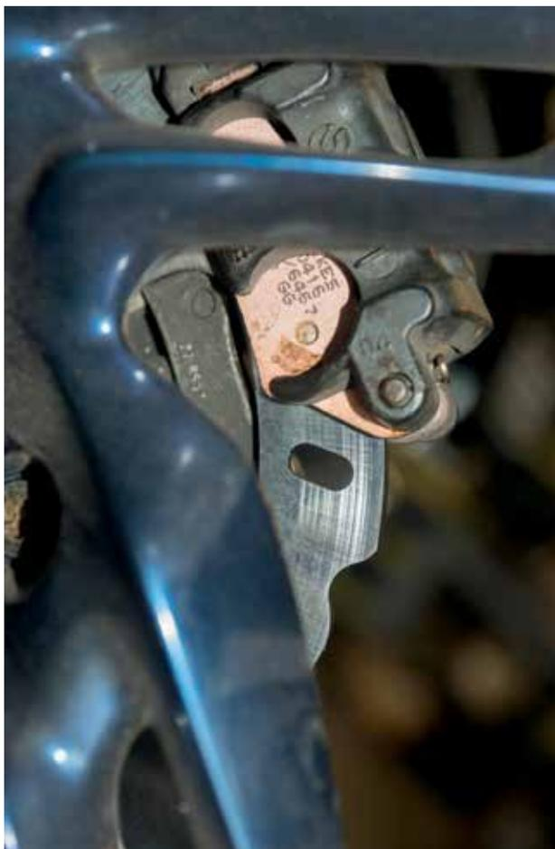
This rear view of the Wave brake rotor shows the contoured outer edge and one of the cutouts that helps cool and clean the pads.
