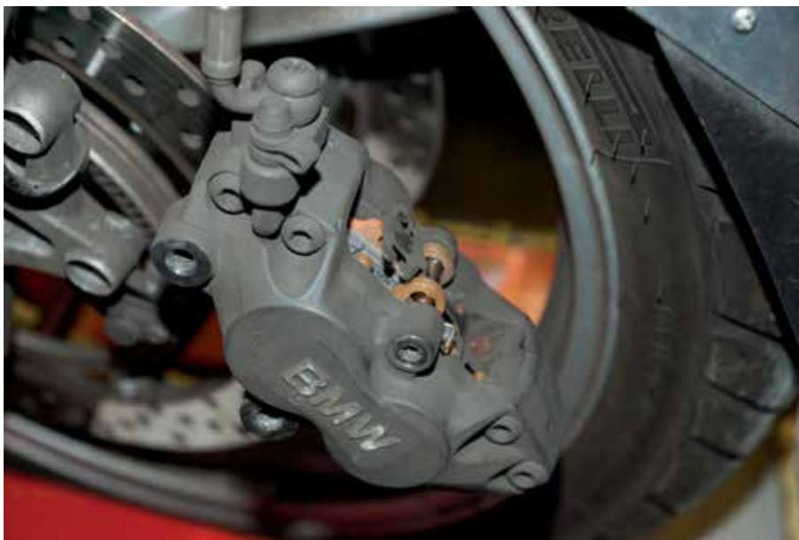
The thin metal arm that fits into the caliper and over the pads keeps pressure on the pads and prevents them from vibrating, thus cutting down on noise.
