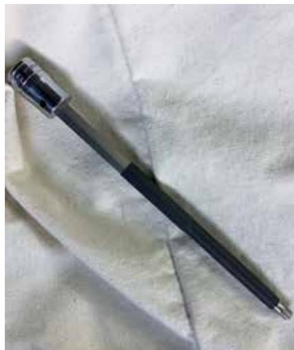
Modified long-necked T40 bit for the bolts on the rear rotor. It's not an absolutely necessary tool, but it makes the job easier.
