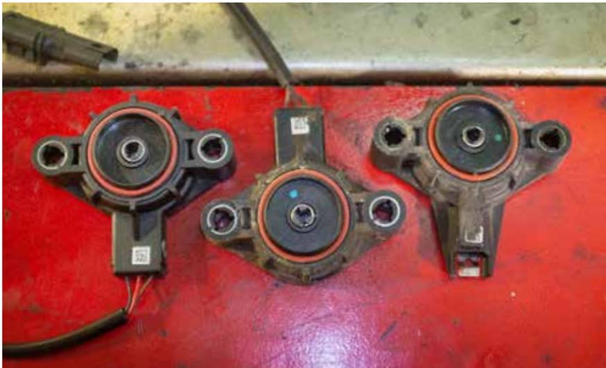
From left to right – new pot with D-shaped hole; pot with T-shaped hole; old pot with D-shaped hole. Note that the old pot lacks wires, while the new pot has them. The excess wiring needs to be carefully zip-tied and tucked out of the way next to the starter.
