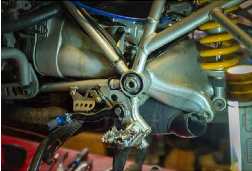
Use the ground-down 30mm socket to loosen the lock nut on the left pivot shown here a few inches above the foot peg. After you remove the right pivot, you can remove the lock nut and the left pivot, which requires a 12mm hex tool. Support the weight of the swing arm for easier removal.
