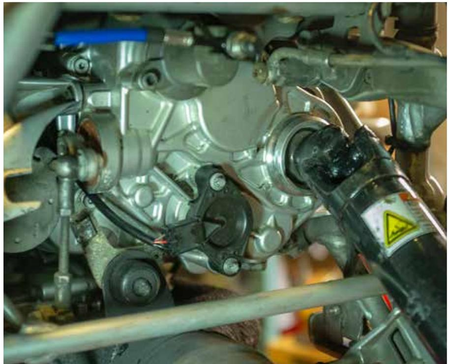
The gear position potentiometer is just to the left of the drive shaft, held in place with one electrical connection and two E8 (external Torx) bolts.
