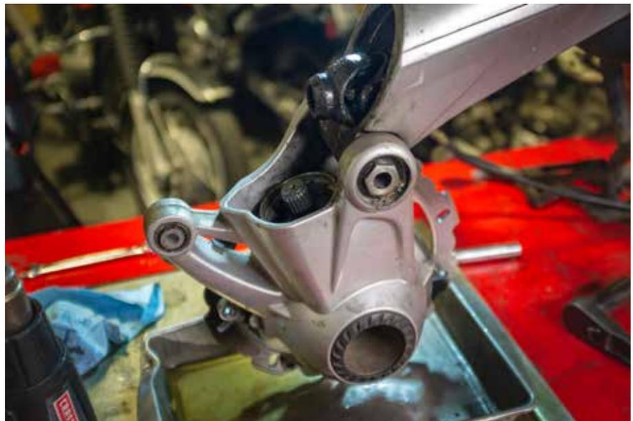
Go ahead and drain your final drive before removing it – it's going to lose fluid through the fill hole anyway, so just be prepared with the required amount of the required oil and a catch pan.
