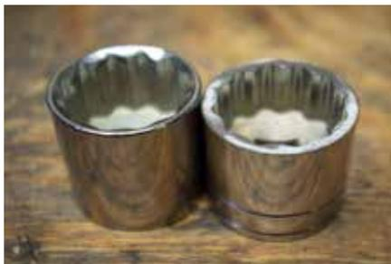
Grind the top eighth of an inch or so off a 24 and 30mm socket (30mm shown here) to make removing the swing arm easier.
