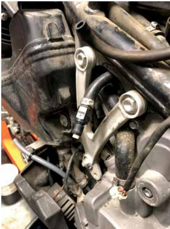
KTM uses the same cheap fuel line quick disconnects (**above**) that BMW uses. With an all-plastic design and an o-ring exposed to shearing forces any time the two parts are connected, it's easy to damage or break these units. Replacing them with Jiffy-Tite quick disconnects (**below**) puts machined aluminum where plastic used to be and ups not only the design quotient, but also the security of knowing you won't wreck the part simply by using it.
