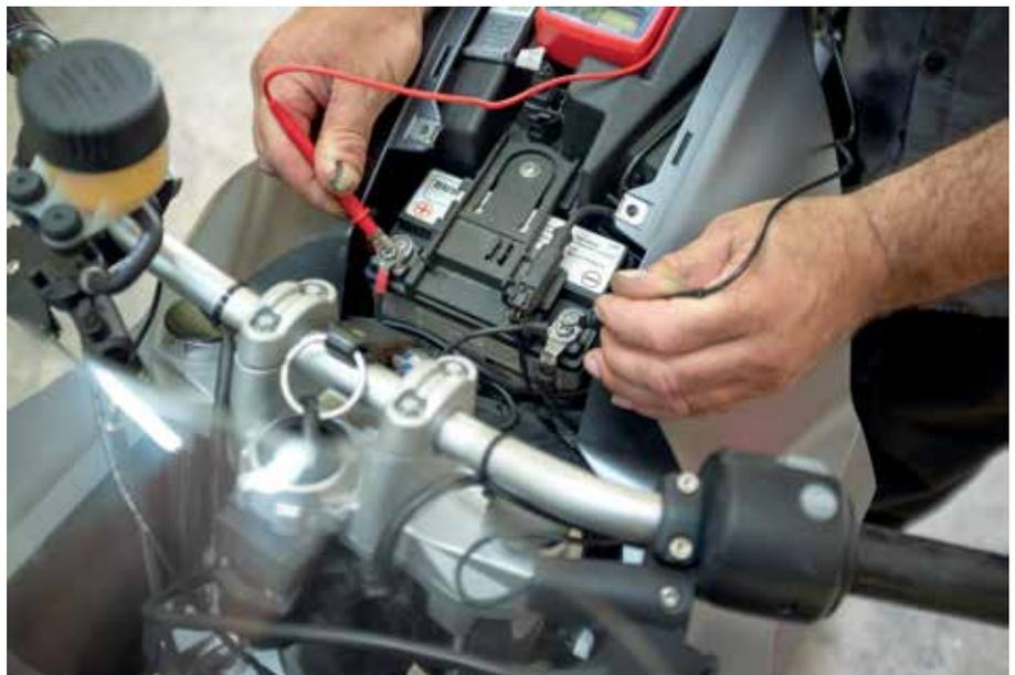
To test your battery, plug the leads into your multimeter. The Common socket on the meter (marked "COM") is for the negative (black) lead. For the positive (red) lead, you may have a single socket choice, which makes it easy, or you may have to choose between two possible sockets. Consult your multimeter's instructions to be sure which to use. Then hold the metal tips of the leads—called "probes" for obvious reasons—against the appropriate terminals of the battery.
