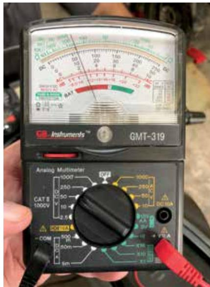
Analog multimeters (AVOM) are more difficult to read quickly and generally bulkier than digital meters, so they're often best suited for home or garage use, rather than sticking them in your road tool kit. This GB Instruments GMT-319 features seven functions including a good/bad battery tester and can handle up to 1,000 volts.
