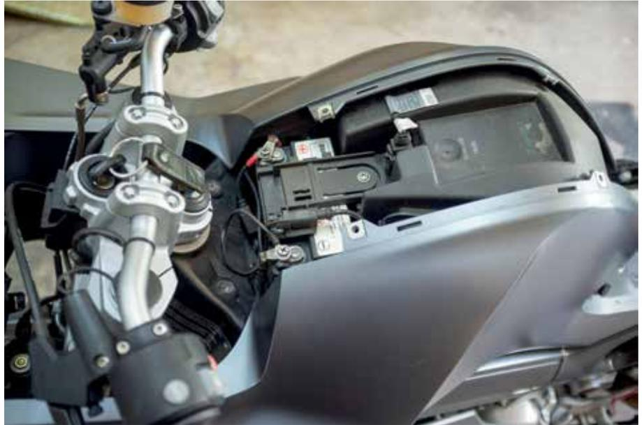
On an F 800 ST, the battery is easy to access. Remove the seat, take out the eight fairing screws holding the center panel in place, and there it is under the center panel.
