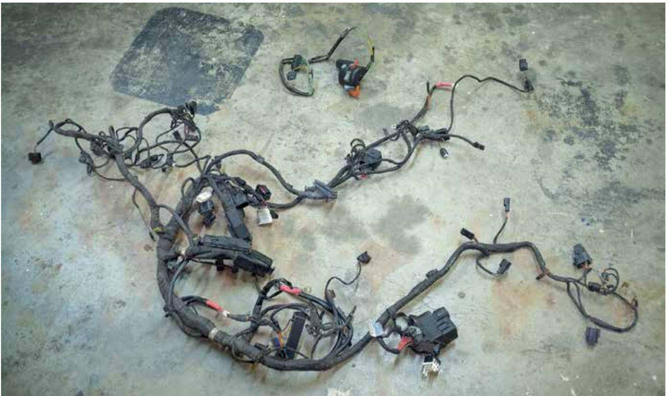
The wiring harness of a motorcycle – such as this one from an R 1150 RTP – can be considered the spinal column of the electrical system. The connectors hook up to various components and transmit power and data as needed to everything on the motorcycle.
