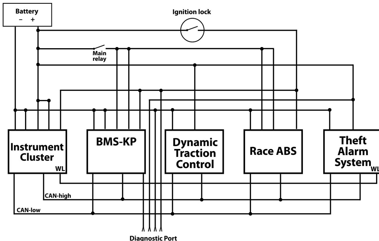
This is a simplified illustration of some of the ECUs on a 2010 S 1000 RR. A number of things are left out, such as fuses, relays, resistors, connectors and other things in the circuit. The purpose here isn't to give a comprehensive look at the wiring of an RR, but rather to show the interconnectedness of the CAN bus system and how all the ECUs communicate with each other.
